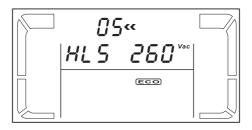
Parameter 2 & 3: Set the acceptable high voltage point and low voltage point for ECO mode by pressing the Down key or Up key.
