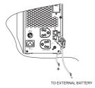
Please refer to below picture to secure battery cable to the terminal with supplied screws and nuts.
