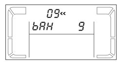
Parameter 3: Set up total battery AH value of the UPS. (unit: AH)
