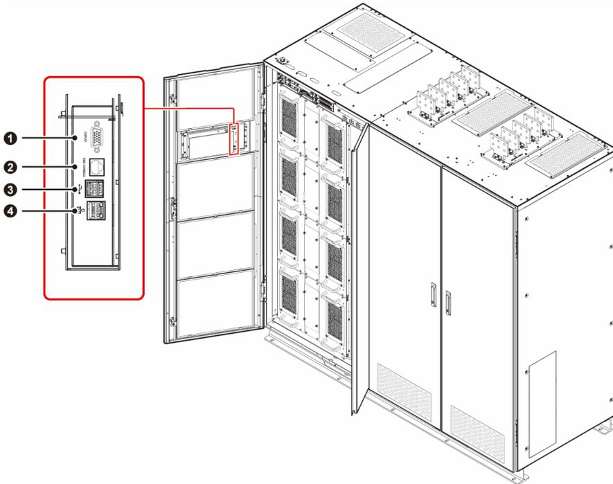
(Figure 4-9: Communication Interfaces (II): at the Rear of the Touch Panel)
