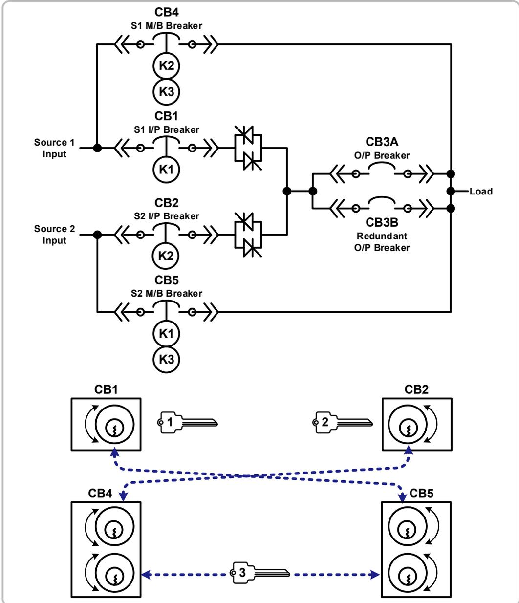
(Figure 6-1: STS One-line Diagram & Kirk-key Interlock Operation)
