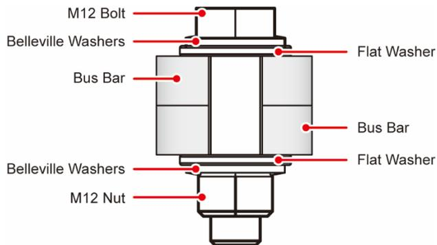
**(Figure 5-6: Installation of the Provided Bolts, Nuts, Flat Washers & Belleville Washers)**
