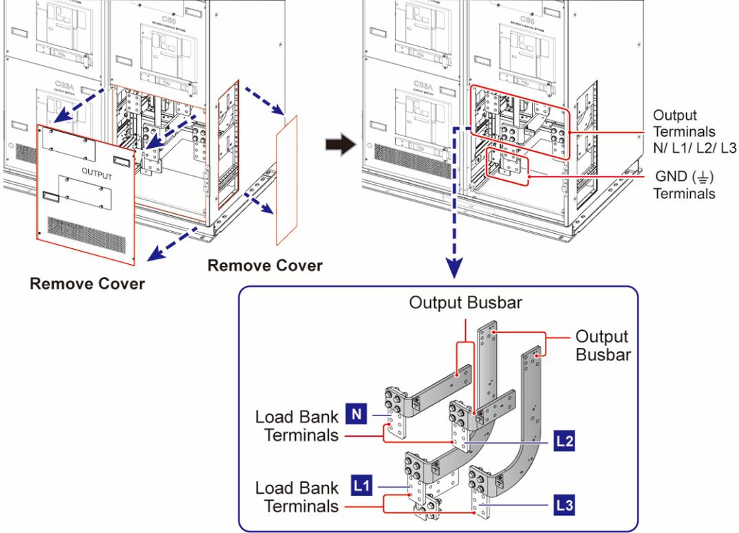
(Figure 2-5: Wiring Terminals\_ Front Side)
