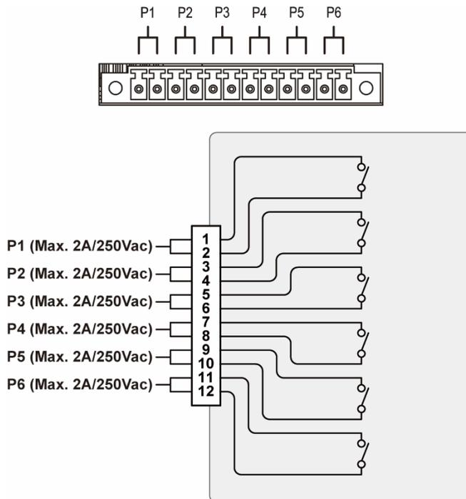
(Figure 4-3: Output Dry Contacts & Schematic)
