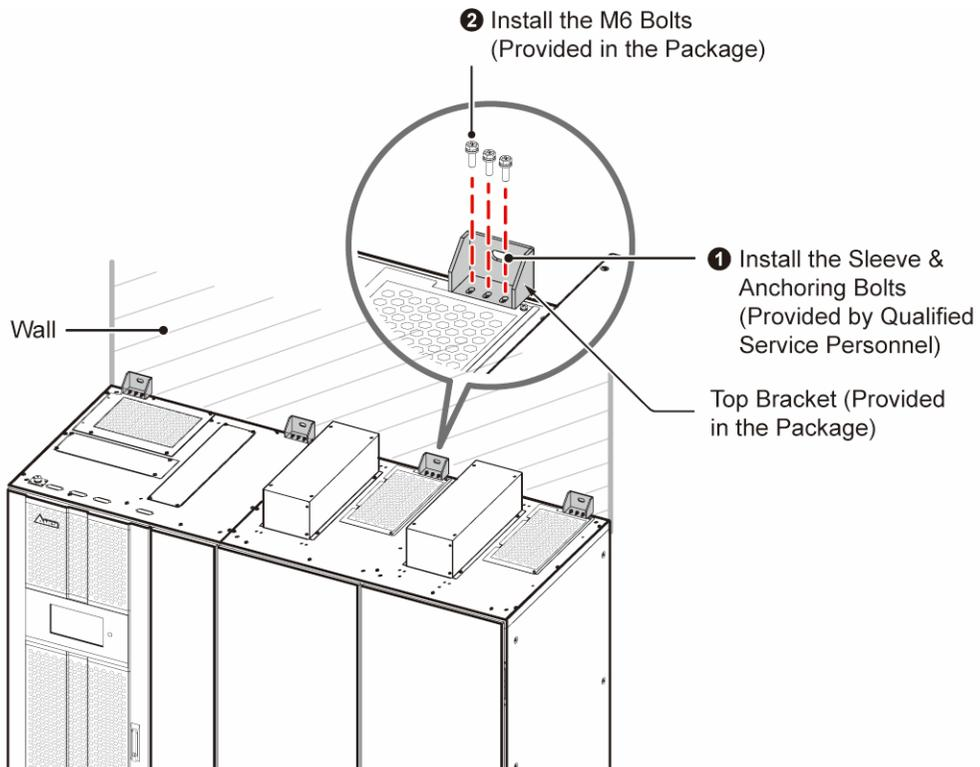
(Figure 5-5: Install the STS against the Wall)
