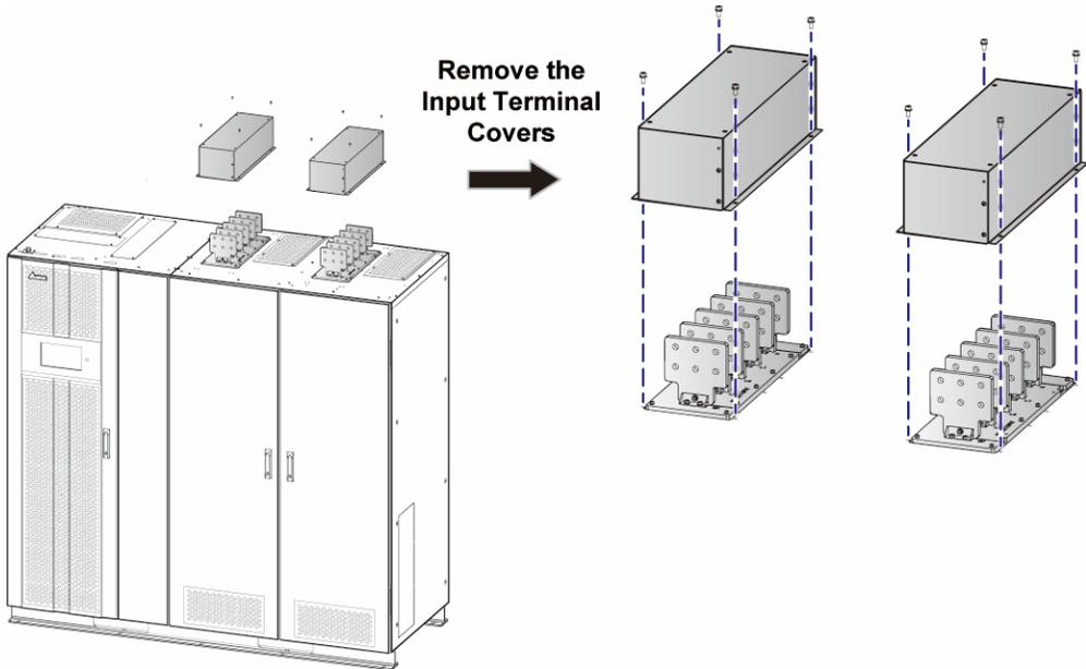
(Figure 5-7: Top Cable Entry\_ for the Input Source)
