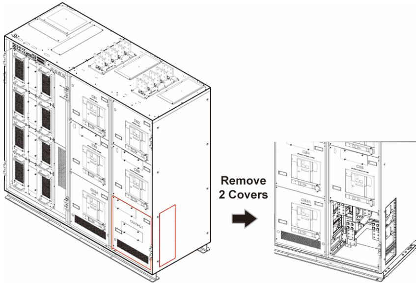
(Figure 5-8: Bottom Cable Entry\_ for the Output Source)
