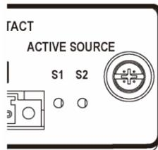
(Figure 4-5: Active Source LED Indicators (S1/ S2))
