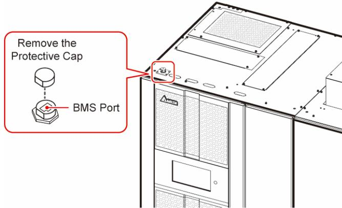
(Figure 4-7: BMS Port on the Top of the STS)
