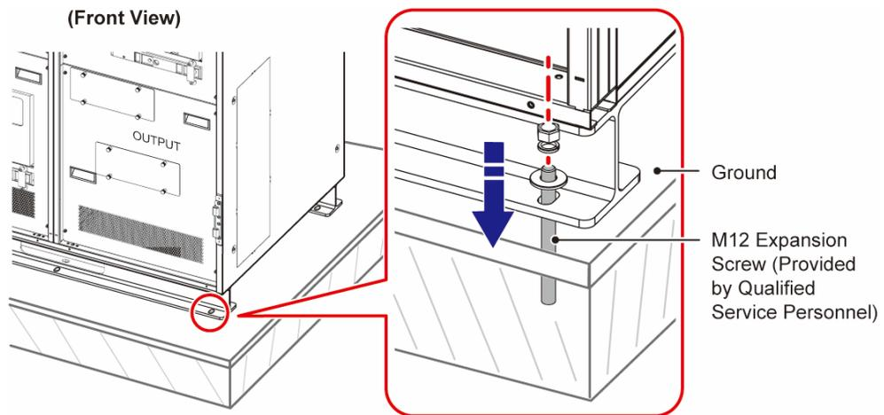
**(Figure 5-3: Fix the Stands on the Ground)**
