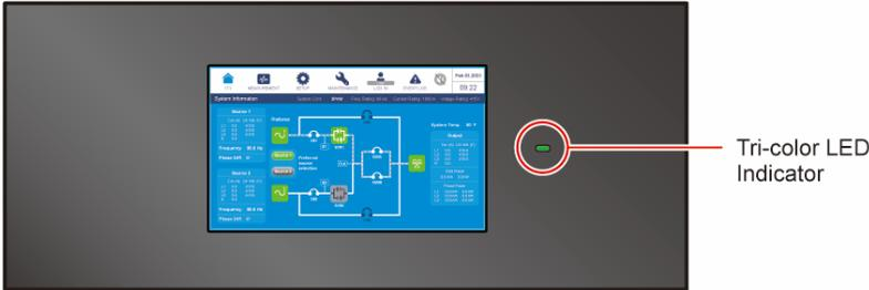
(Figure 2-7: Tri-color LED Indicator Location)
