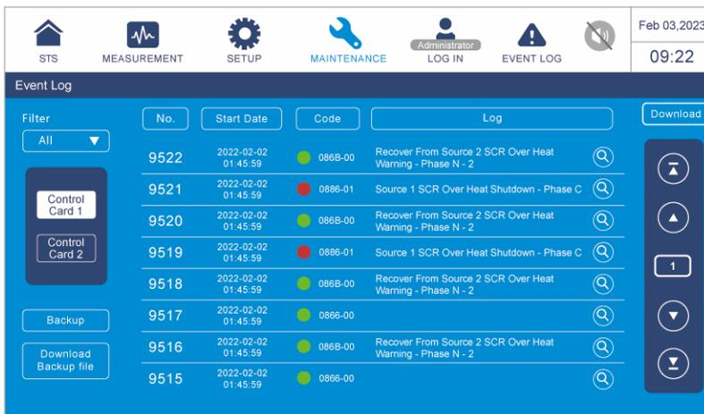
The screen shows the control card 1 and control card 2's event logs. Refer to the table below for button information.
