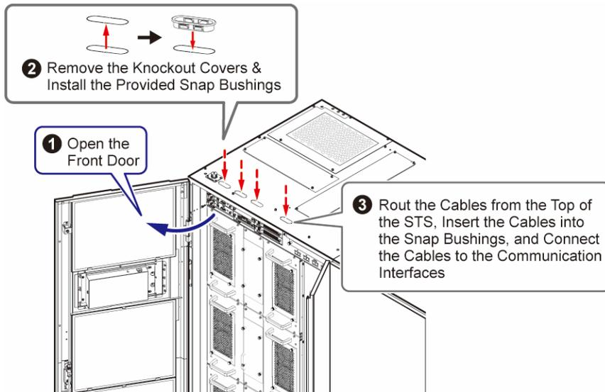
(Figure 4-10: Top Cable Entry for the Communication Interfaces)
