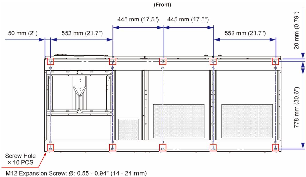
(Figure 5-2: Cabinet Floor Fixing Points)
