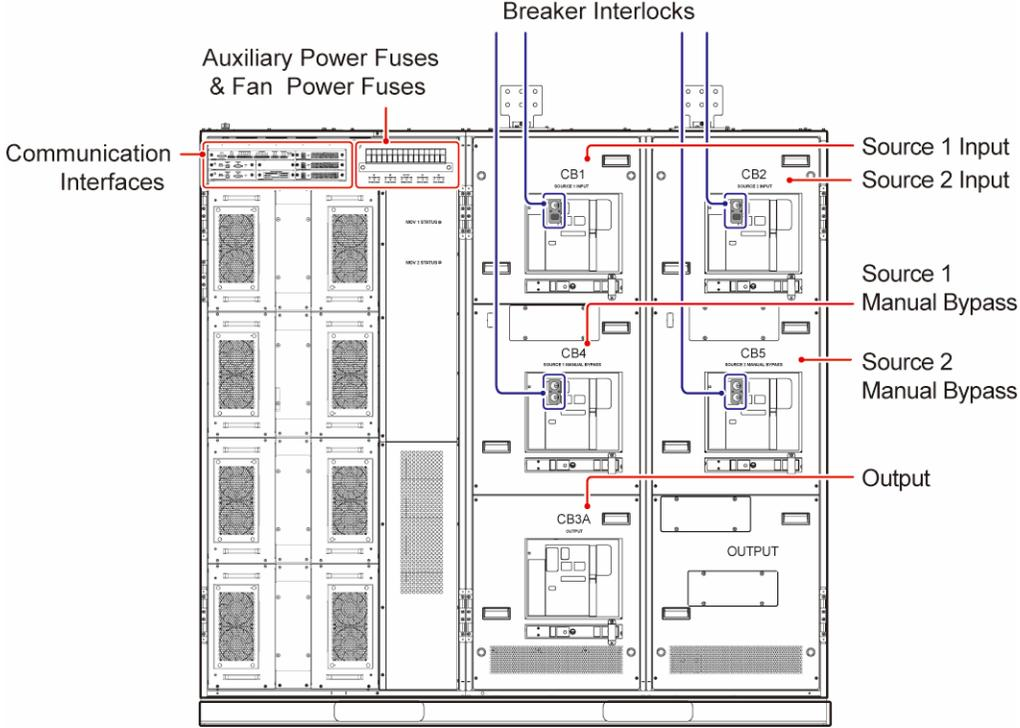
(Figure 2-4: Internal View with Front Doors Open)
