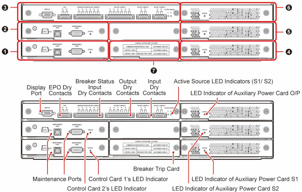
**(Figure 4-1: Communication Interfaces (I): on the Front of the STS with its Front Door Open)**
