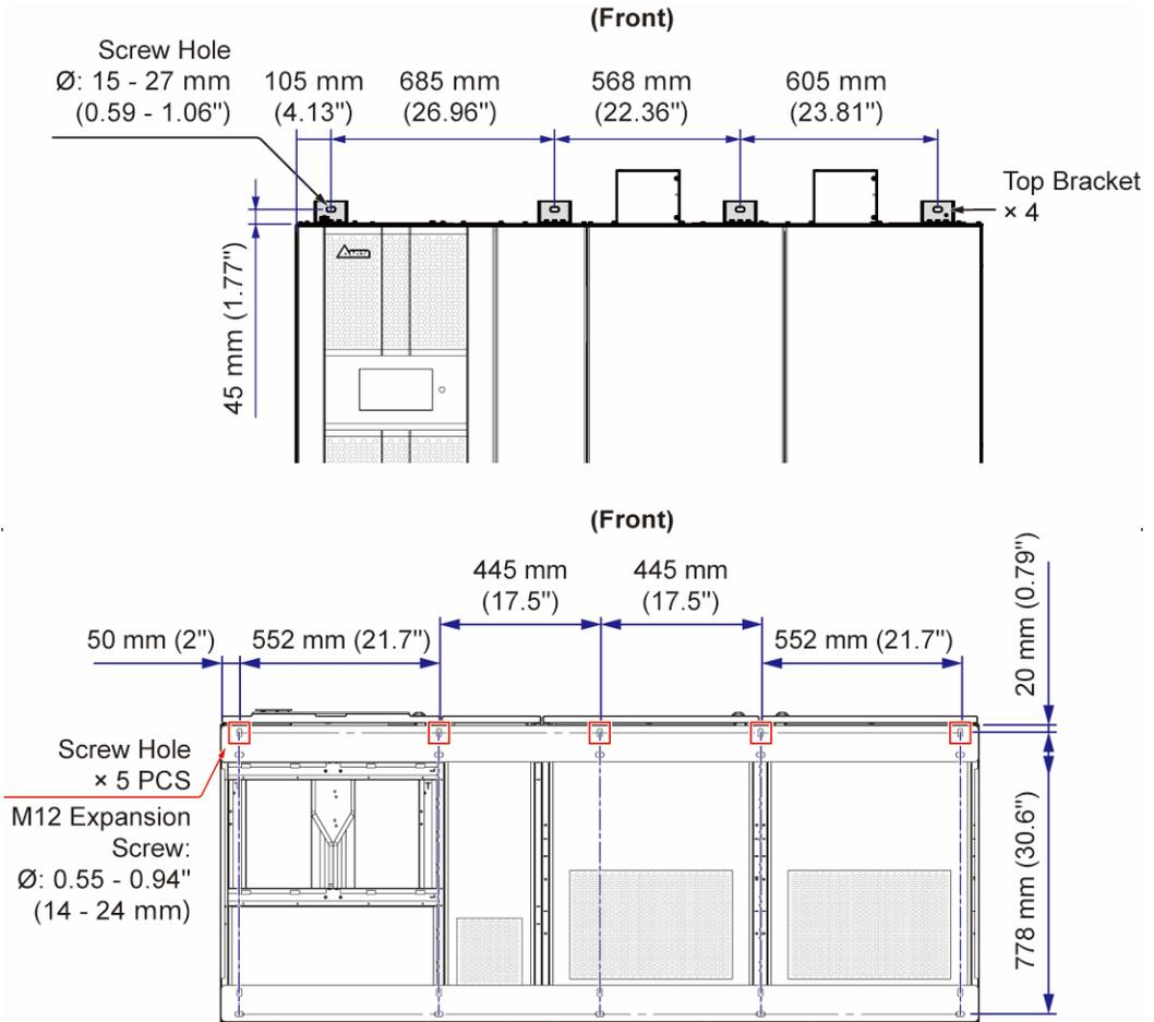
**(Figure 5-4: Wall Fixing Points)**
