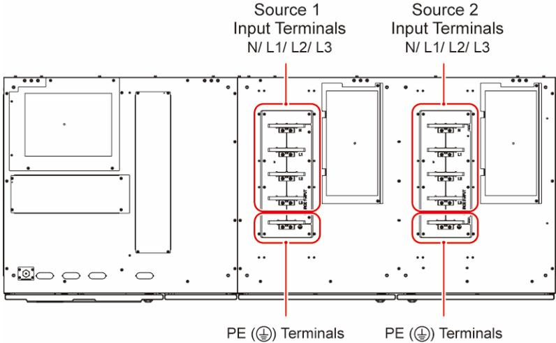
(Figure 2-6: Wiring Terminals \_ Top View)
