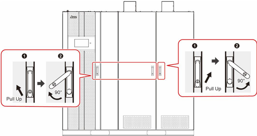
(Figure 2-3: How to Open the Front Door)
