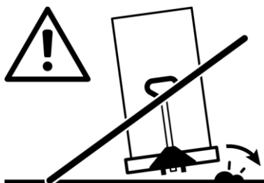
Figure 5-2: Clear All Obstacles from the Transportation Route
