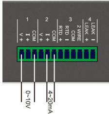
The Analog Input 3 is dedicated to a 2-wire or 3-wire RTD (Resistance Temperature Detector) input. You can connect a PT100 (2/3-wire) temperature sensor to it. Please see the figure below:
