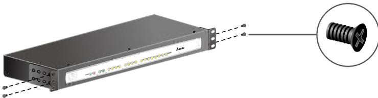
**Step 3** Make sure the mounting holes and the bracket ears on the EnviroStation are aligned properly, then secure the bracket ears to the rack with the four provided mounting screws (two for each end), EnviroStation occupies 1U of rack space.
