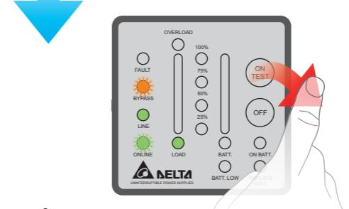
**EN** When you hear the beep, immediately release the ON/TEST button!
