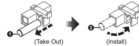
3 Replace the fuse cover back to the rear panel.
