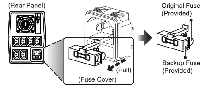
2 Replace the original fuse 1 with the provided backup fuse 2.
