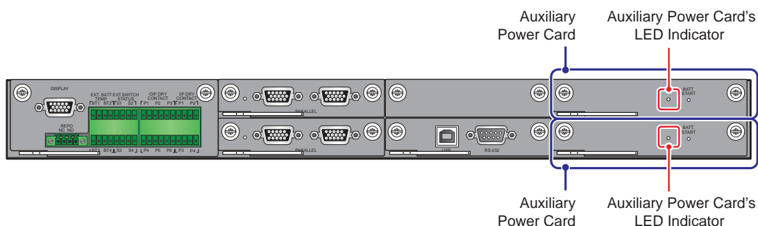
(Figure 4-15: Location of the Auxiliary Power Cards)
