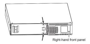
A Remove the metal top cover of the battery box by unscrewing the 8 screws present on the two sides (4 on the right side and 4 on the left side), 3 screws on the top and 4 screws on the back side.
