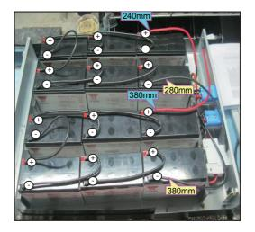
**NOTE:** The cable connection from external battery connector to PCB is already present inside the battery box. All the other cable connection should be followed by wiring diagram.
