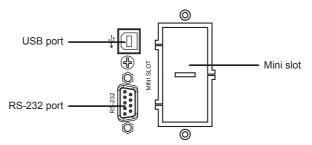
To allow for unattended UPS shutdown/ start-up and status monitoring, connect the communication cable one end to the USB/ RS-232 port and the other to the communication port of your PC. With the monitoring software installed, you can schedule UPS shutdown/ start-up and monitor UPS status through PC.
