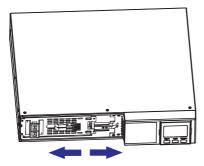
3 Pull out the battery box by removing the two screws on the front panel.
