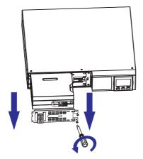
A Remove the top cover of the battery box and replace the inside batteries.
