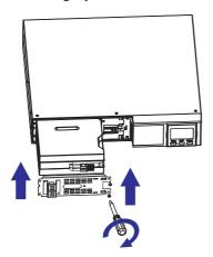
**6** Re-connect the battery wires.
