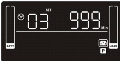
**Parameter 2:** Set up backup time limits for programmable outlets.
