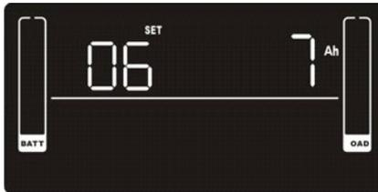
**Parameter 2:** Set up the battery total AH of the UPS.
