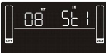
**Parameter 2:** Set Input Waveform Sensitivity.
