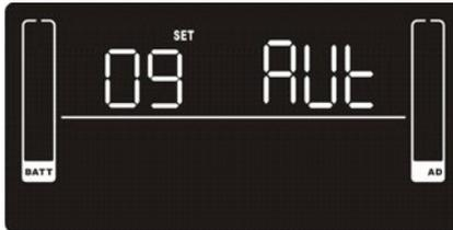
**Parameter 2:** Set up the working mode for the LCD display backlight.
