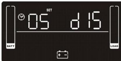
**Parameter 2:** Set up backup time on battery mode for general outlets.
