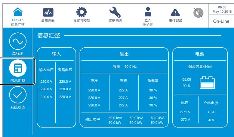
The screenshot shows the information summary screen. At the top right, the time is 09:30, date is May 10, 2018, and status is On-Line. The main area is divided into three sections: '输入' (Input), '输出' (Output), and '电池' (Battery).
