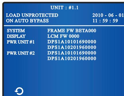
The firmware version screen above shows you the system, display and power unit's firmware versions.
