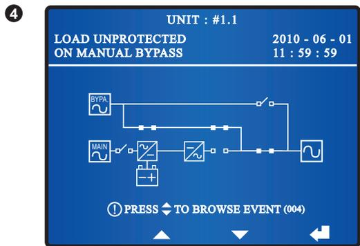
When the screen above appears, it means that the UPS is in bypass mode. If the bypass AC source fails, the critical loads won't be protected.
