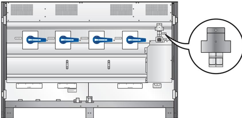
(Figure 7-1: Close the Auxiliary Power Fuse Holder)
