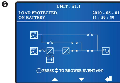
When the screen above appears, it means that the UPS is in battery mode.
