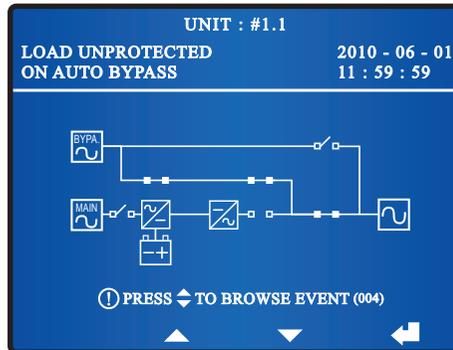
The nine statuses of the UPS shown in the LCD display are as follows.
