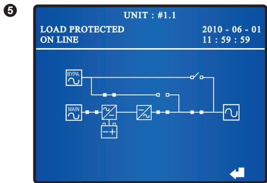
When the screen above appears, it means that the UPS is in normal mode.
