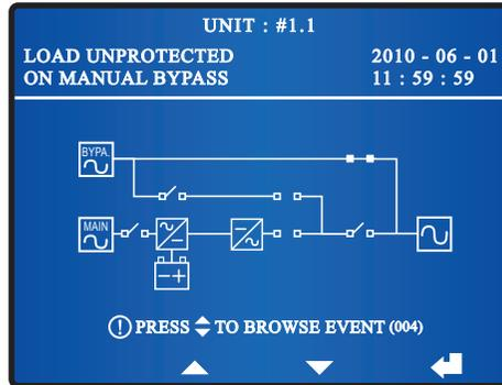
When the screen above appears, it means that the UPS is in manual bypass mode. Before maintenance, do not forget to switch the UPS into manual bypass mode and cut off the main AC source and batteries. During this mode, if the bypass AC source fails, the critical loads won't be protected.
