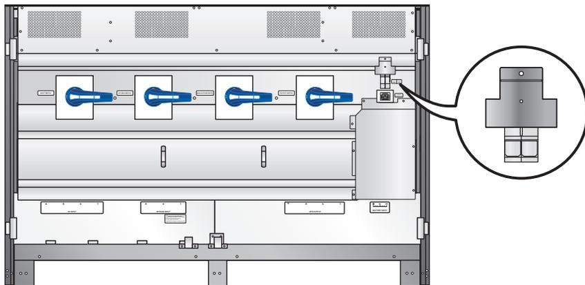
(Figure 7-2: Close the Auxiliary Power Fuse Holder)
