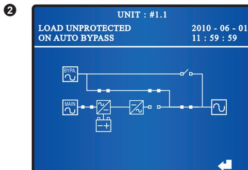
When the screen above appears, it means the bypass is supplying power to the critical loads.
