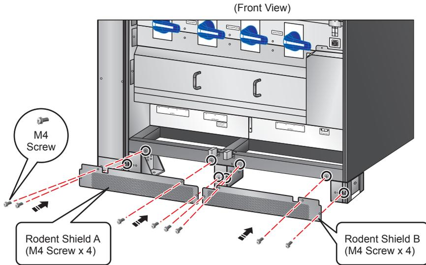
**(Figure 6-4: Install the Rodent Shields A & B at the Front of the UPS)**
