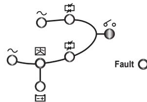
The status of the LCD and LEDs for the remaining parallel UPSs:
