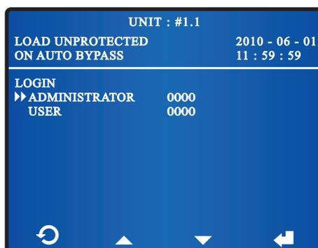
If an interval between settings is over five minutes, you have to login and enter the password again. If the password is wrong, the system will go back to the screen that you have selected the item for setup change.
