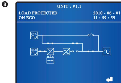
When the screen above appears, it means that the UPS is in ECO mode and the bypass supplies power to the critical loads. Please see **8.7.2 Output Setup** for ECO mode setup.
