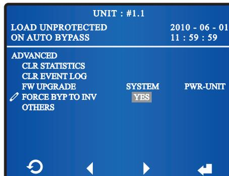
Use the function keys below the symbols '◀' and '▶' to select 'YES' or 'NO'. Once you select 'YES' and press the function key below the symbol '◀', the system will transfer from bypass mode into inverter mode. The administrator password is required.
