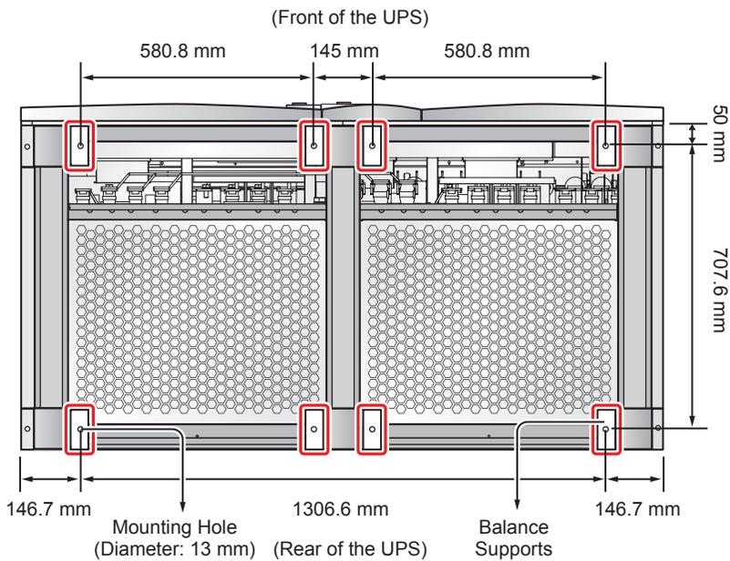
(Figure 5-2: Mounting Hole Diagram)
