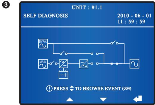
When the screen above appears, it means that batteries have started up the UPS.
