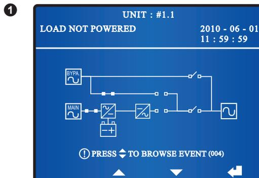
When the screen above appears, it means that no power is supplied to the critical loads connected.
