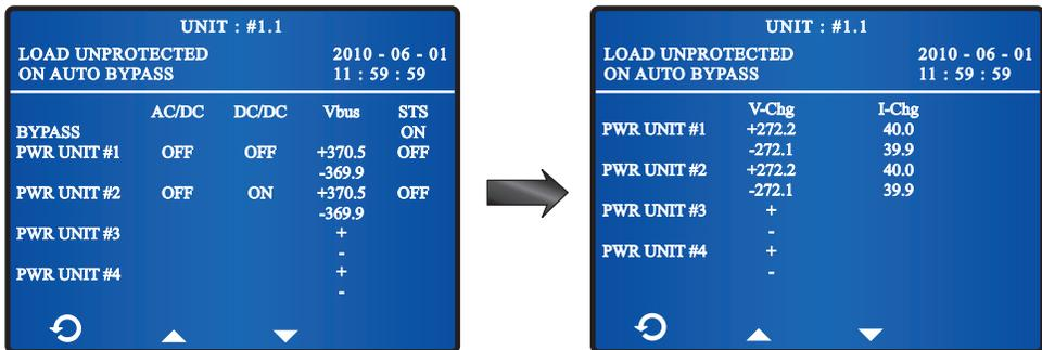
AC/DC & DC/DC, Vbus, STS, V-Chg, and I-Chg mean PWR UNIT #n PFC status, DC bus voltage, static switch status, charge voltage and charge current respectively.
