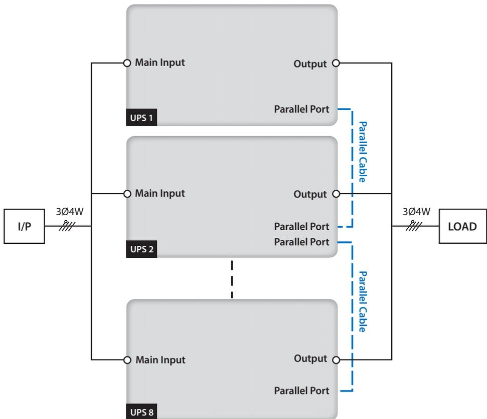
(Figure 5-15: Parallel Units Single Input Wiring Diagram)
