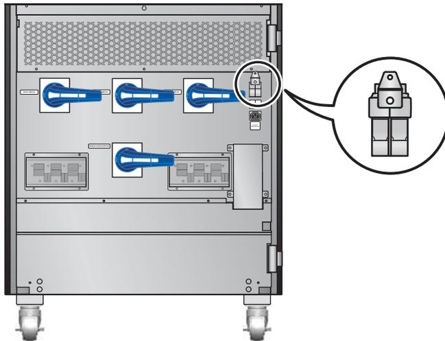
(Figure 6-1: Close the Auxiliary Power Fuse Holder)
