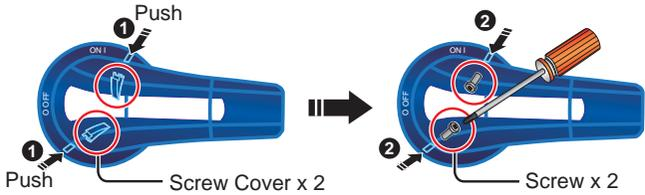
(Figure 5-8: How to Remove a Switch)
