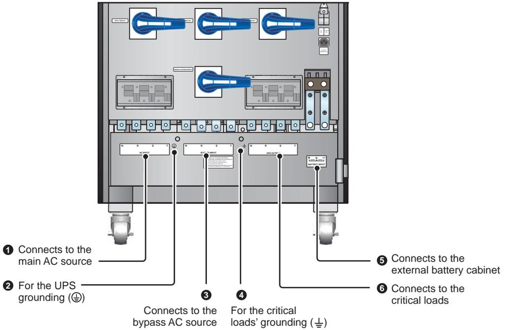
(Figure 5-11: Wiring Terminal Block)
