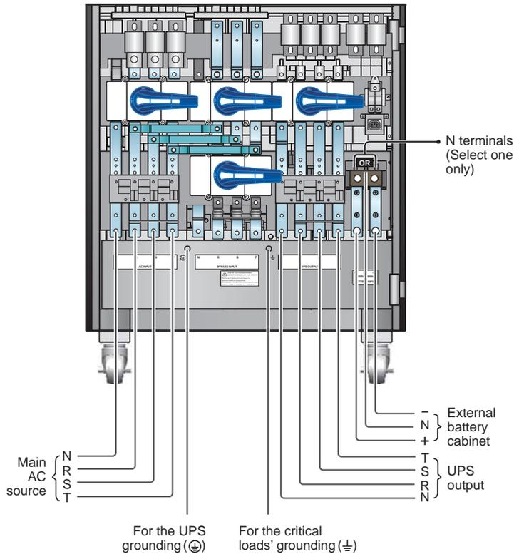
(Figure 5-13: Single Unit Single Input Wiring Diagram)
