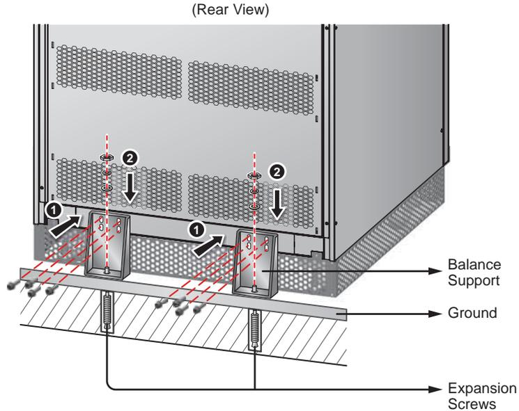
(Figure 5-4: Install the Balance Supports at the Rear of DPS)
