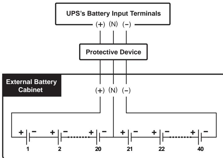
(Figure 5-17: External Battery Cabinet Connection)
