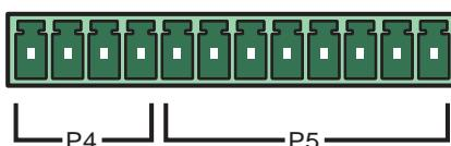
(图 4-7：外接电池箱干接点)
