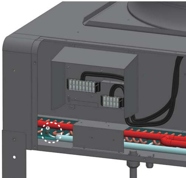
(Figure 3-23: Outdoor Unit Refrigerant Service Valve)
