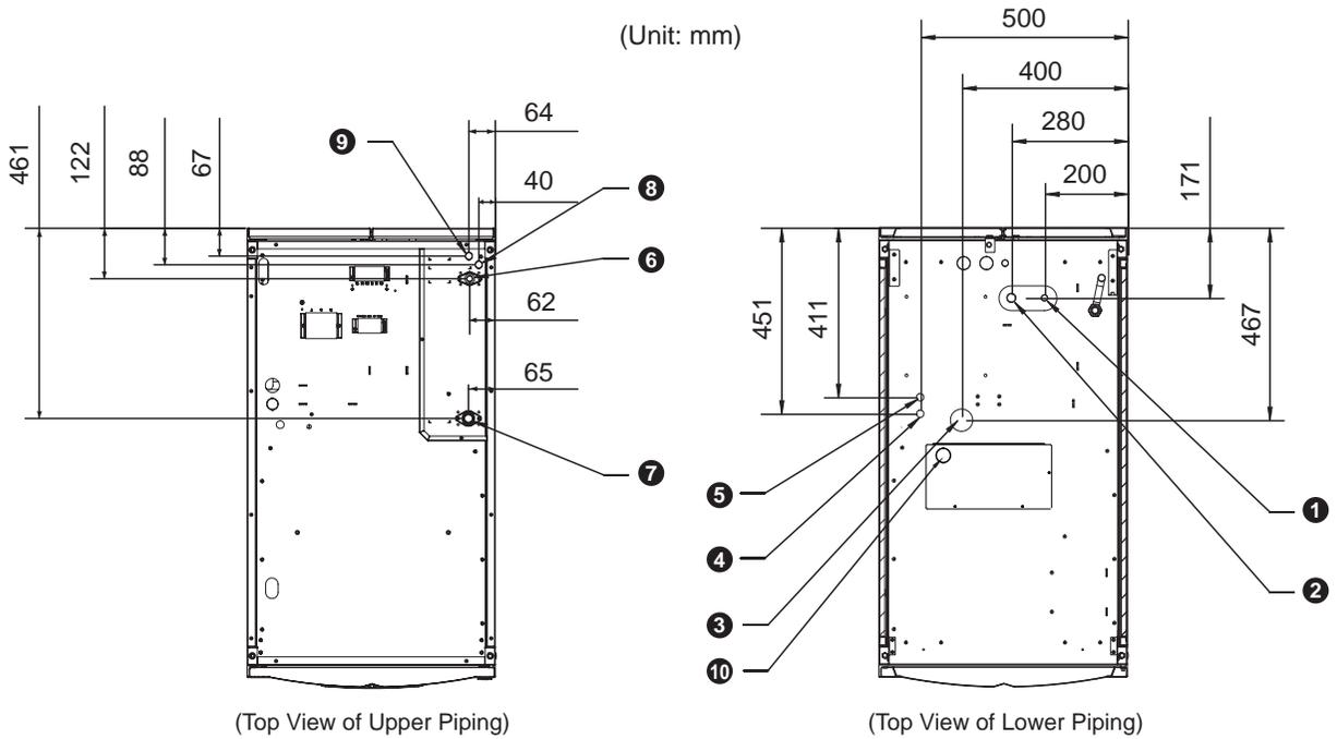
**(Figure 3-12: Location & Dimension Drawing of Upper & Lower Piping)**
