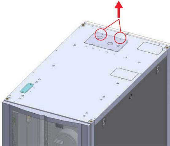
*(Figure 3-15: Remove the Power Supply Cover)*
