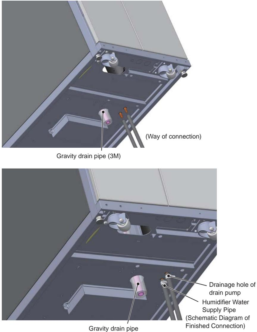
**(Figure 3-14: Drain Pump & Humidifier Water Supply Pipe)**
