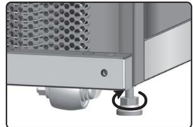
(Figure 3-6: Rotate Each Leveler Clockwise)
