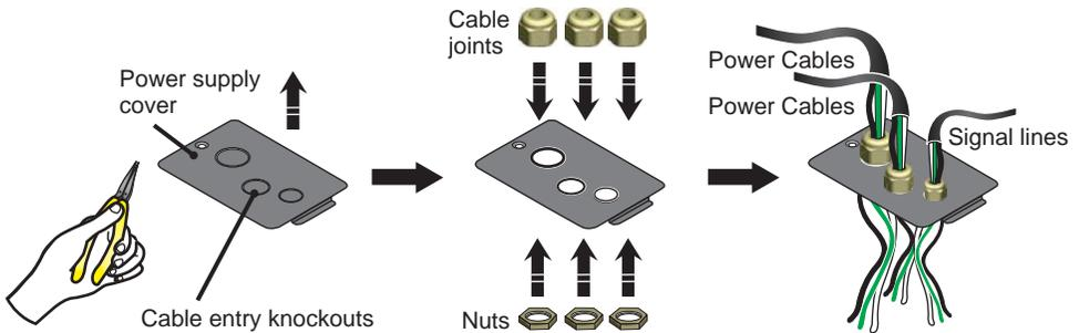
*(Figure 3-16: Insert the Power Cables & Signal Lines)*
