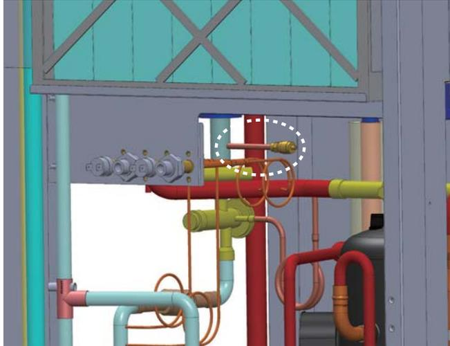
(Figure 3-24: Indoor Unit Refrigerant Service Valve)
