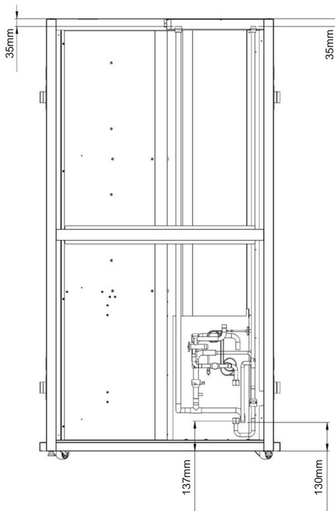
(Figure 3-11: Location & Dimension Drawing of Upper & Lower Piping)
