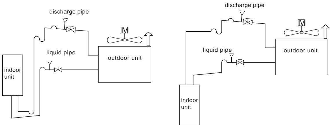
(Figure 3-13: Recommended External Pipeline)
