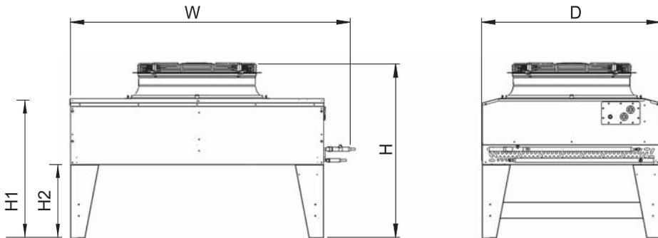
(Figure 2-2: Appearance & Dimensions of Outdoor Unit)
