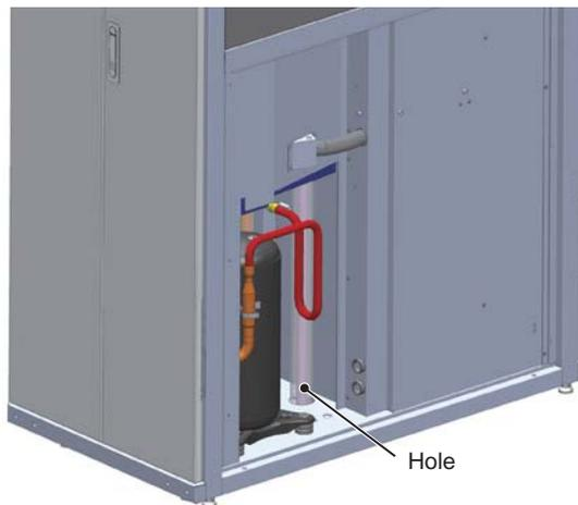
(Figure 4-5: Installation of Water Leakage Detection Cable)
