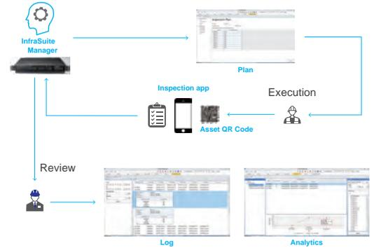
FIGURE 7. The flow of Inspection Execution and Review
