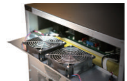
Redundant fan design enhances system reliability*
