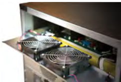
Redundant fan design enhances system reliability
