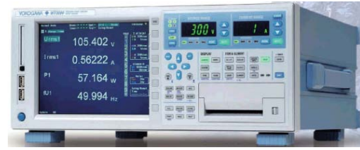
Fig.1 Power analyzer (Yokogawa, WT3000)
