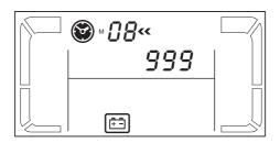
Parameter 3: Set up backup time in battery mode for general outlets.
