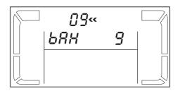
Parameter 3: Set up total battery AH value of the UPS. (unit: AH)
