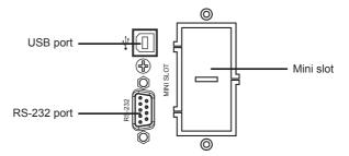
To allow for unattended UPS shutdown/ start-up and status monitoring, connect the communication cable one end to the USB/ RS-232 port and the other to the communication port of your PC. With the monitoring software installed, you can schedule UPS shutdown/ start-up and monitor UPS status through PC.
