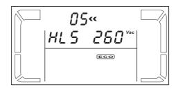
**Parameter 2 & 3:** Set the acceptable high voltage point and low voltage point for ECO mode by pressing the Down key or Up key.
