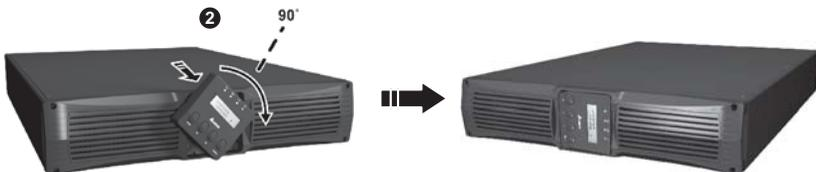
(Figure 4-4: Rotate the UPS Control Panel)
