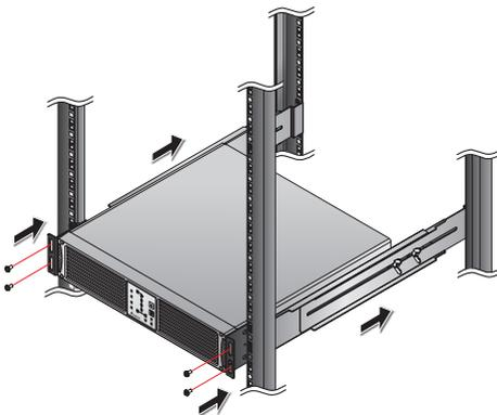
(Figure 3-4: Insert the UPS into Your Rack)
