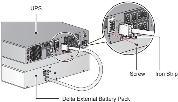
(Figure 4-2 : Connect the UPS and the Delta External Battery Pack )
