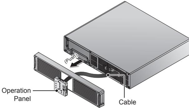
(Figure 3-6: Push the Backside of the Operation Panel)
